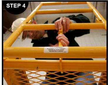
Attach hook end to *inner* telescoping ladder – not outer ladder. TIGHTEN SECURELY
