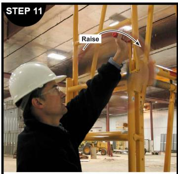
Raise deck to desired height by rotating winch handle in a clockwise direction.
