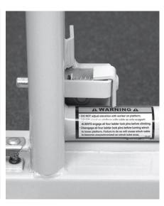
If ladder lock spring pins do not readily engage, raise the cable between the sheaves slightly and jog the telescoping ladder section to help facilitate complete engagement. DO NOT pound on the lock pins.
