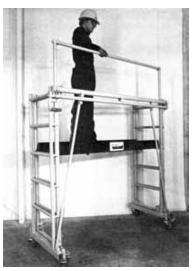
5. For deck heights used that are 6' high or greater, place the deck on the top rungs of the telescoping ladders and attach **ALL FOUR** deck braces between the deck and the base of the telescoping ladders. Jog base of end sections to facilitate brace pin alignment. DO NOT hammer on braces.
