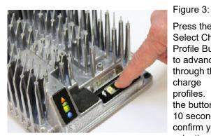
Press the Select Charge Profile Button to advance through the charge profiles. Hold the button for 10 seconds to confirm your selection.
