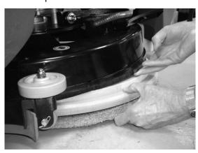
6. Check that release lever/plate is completely closed and pad/brush is securely attached.
