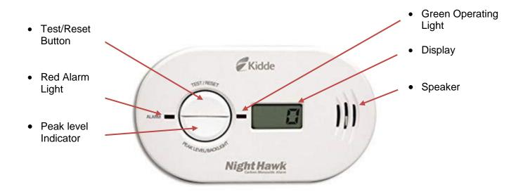
Test the unit monthly by pressing the test/reset button. If the unit is operating properly, you will hear four quick beeps, followed by 5 seconds of silence, followed by four quick beeps. The display will show three "eights" (888) and then show a number, usually around 200. Within several seconds, the unit will return to monitor for CO (display 0).
